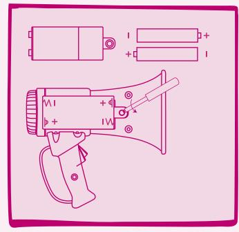
**1.** Open the battery cover with a philips screwdriver. (not included)
