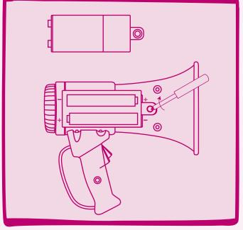
**2.** Install 2 x AAA batteries and follow the polarity orientation, as shown. Close the battery cover with screwdriver.
